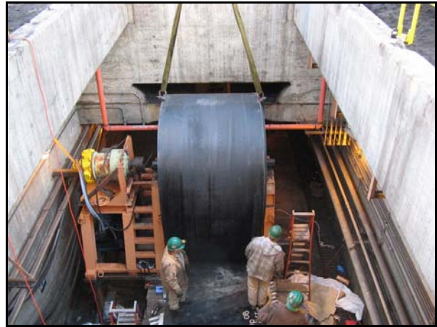
New belt being prepared to go on Conveyor 7.
