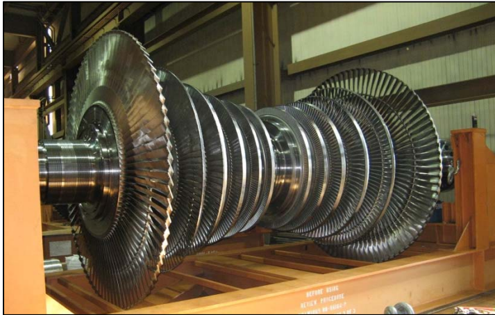
One of the new LP rotors that was installed.
