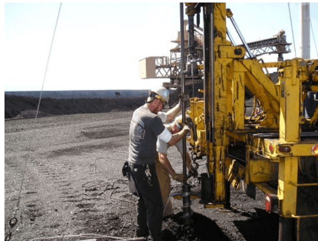
Drilling boreholes into the coal stockpile for measurements.
