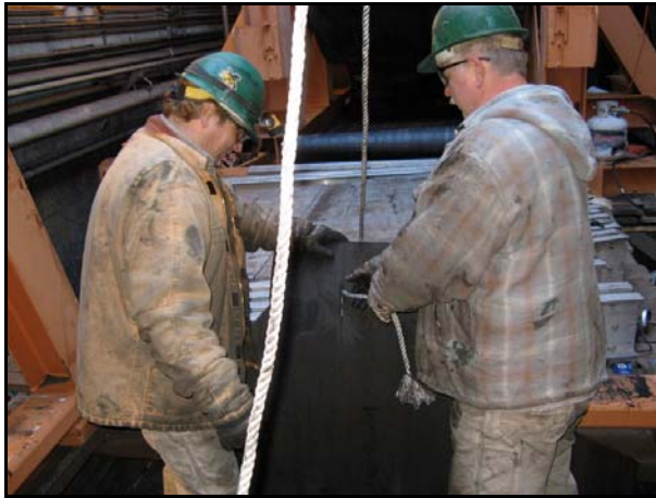
Preparing to feed new belt on rollers.
