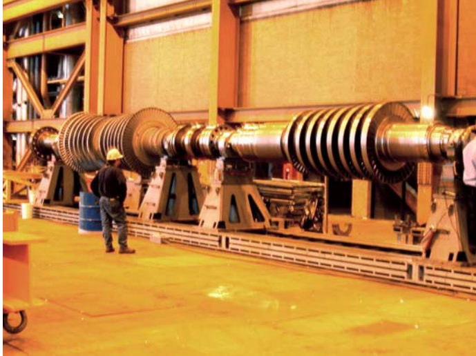
Old turbine alongside the new replacement turbine, the holes of the new turbine will be bored to match the old turbine.
