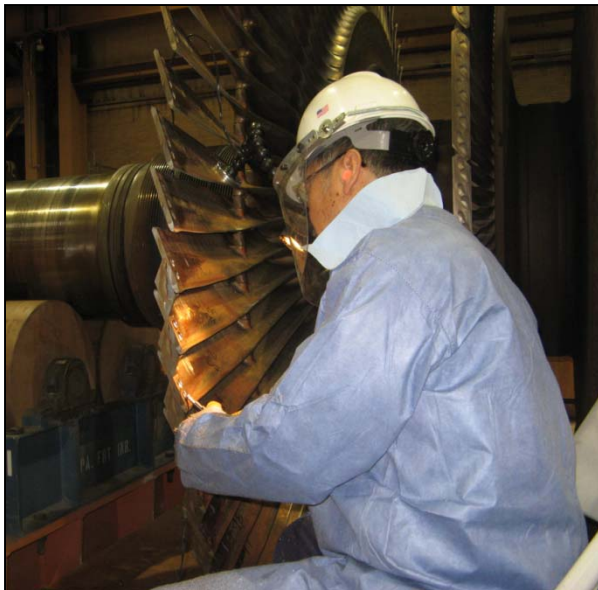
Contractor working on L-0 turbine buckets.
