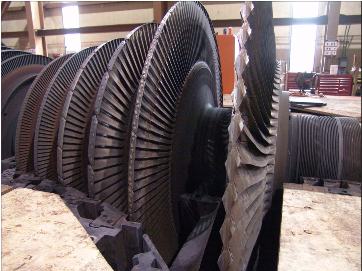
The damaged LP rotor getting ready to have new buckets installed.
