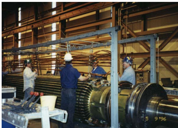
IPSC employees performing a generator field rewind.
