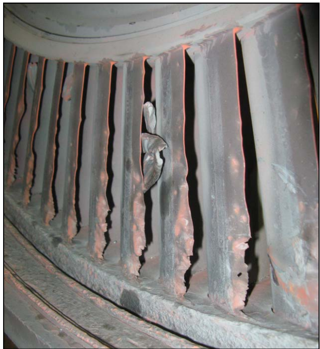
Damaged IP Turbine buckets that were replaced.
