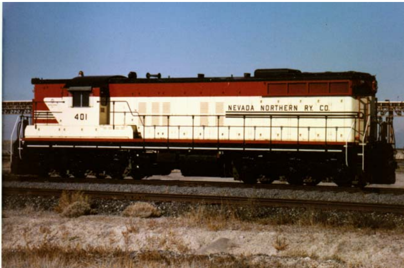
Engine used at power plant to move coal cars, especially useful during winter months to reposition frozen cars.
