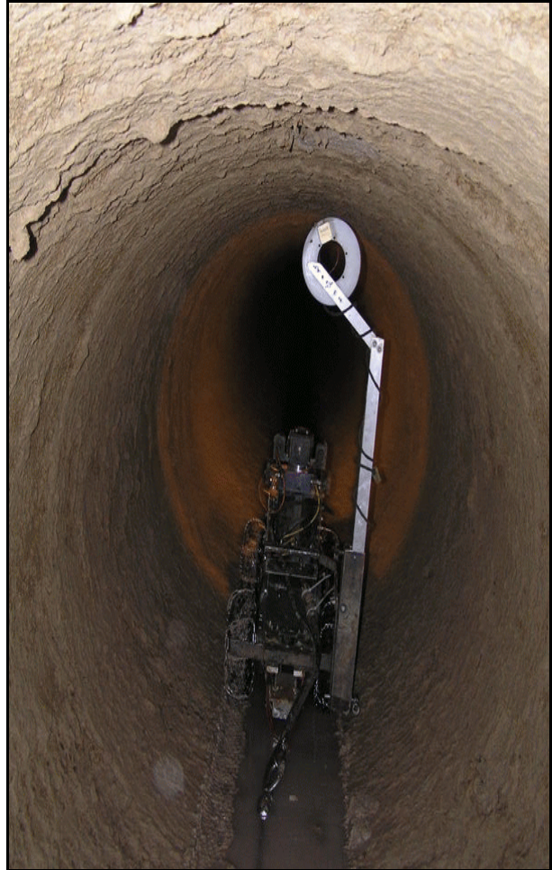
The RFEC/TC inspecting the interior of the DMAD pipeline.
