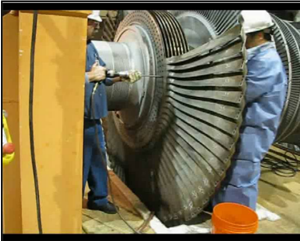
Unit 2 LP Turbine - last stage bucket pin removal on original buckets.
