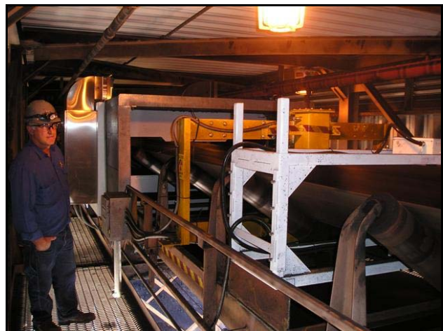
The on-line coal analyzer installed on Conveyor 8.
