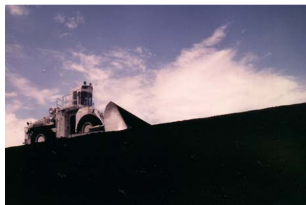
Letourneau used to move coal. The blade is 8 ft. 8 in. high by 24 ft. wide. The tires are 7 ft. 10 in. in diameter.
